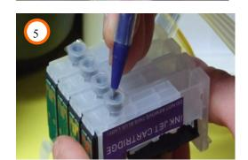
3) Insert the ink in the cartridge until it is filled. (Photo 3).
