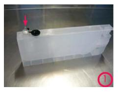
1– In the cartridge back side there are two holes: the big one for the ink refill, the small one for the air. After the refill the small hole must remain open to allow the printer to work correctly.
