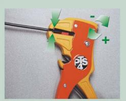
Press on handles; cables il locked by external jaws while the insulation is lightly cut without damaging the conductor.
