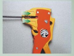
The complete closing of the handles operates a sliding action of the blades that removes the insulation.
