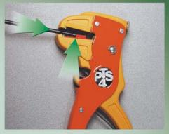
Clamp prepared cable between front blades, against the cablestop, for the lenght to be stripped, using as reference millimeter scales laterally positioned.
