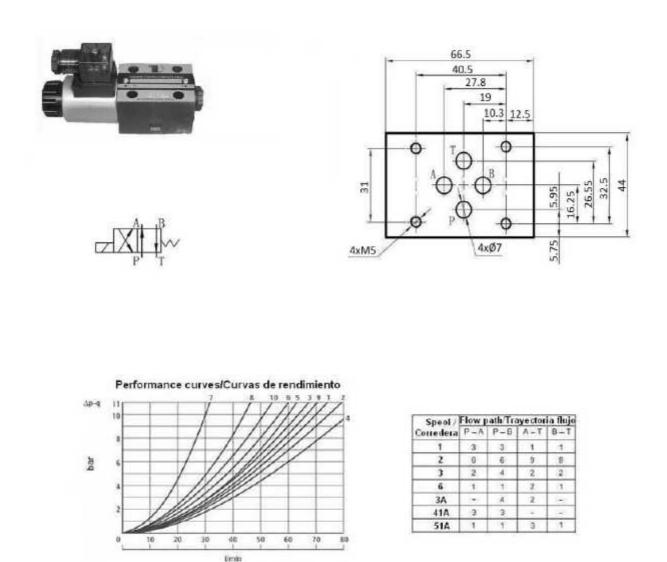
Part nº Max. flow (I/min) f (Hz) Size Voltage (V) Max. Press. (bar) KVNG6-51A-12CC H NG-6 12 VDC 60 315 KVNG6-51A-24CC H NG-6 24 VDC 60 315 KVNG6-51A-110CA H NG-6 110 VAC 60 315 50 KVNG6-51A-220CA H NG-6 220 VAC 60 315 50
