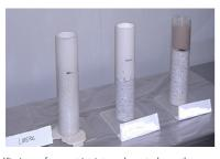
To ensure the **perfect saturation** of small **cracks** or **cavities** and **smaller voids**, we have optimized our formulated that they may have: adequate fluidity, guaranteed by the fineness and purity of the constituents and not through the use of a high quantity of water; absence of bleeding (separation of the liquid phase from the solid one); shrinkage compensated.
